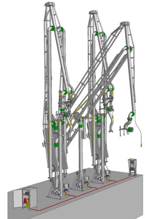
Electric hydraulic control system for more than one MLA
