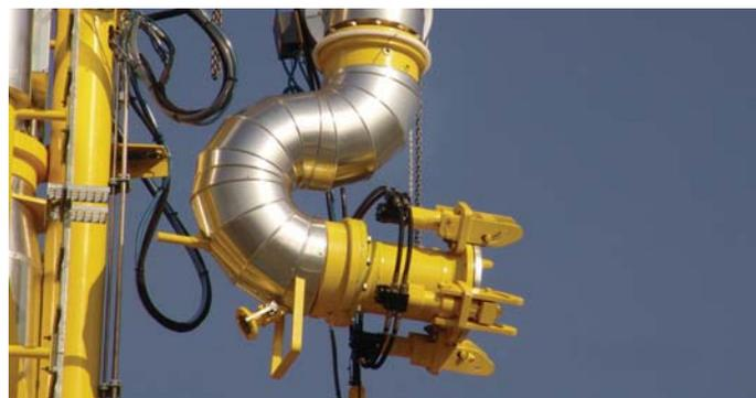
outboard arm, or the line is still pressurised, the operator can get covered up by the contents when disconnecting manually.
